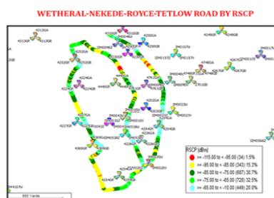
Fig. 1: The log of measurement along Wethederal-Nekede-Royce Tetlow Road.
